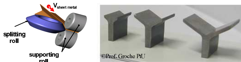
Figure 1: Process principle and produced simple geometry.
