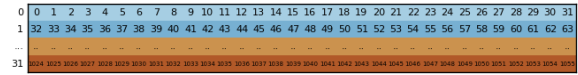
Figure: Compression – each thread reads one data row (colors denote threads, numbers indicate subsequent values in input array)
