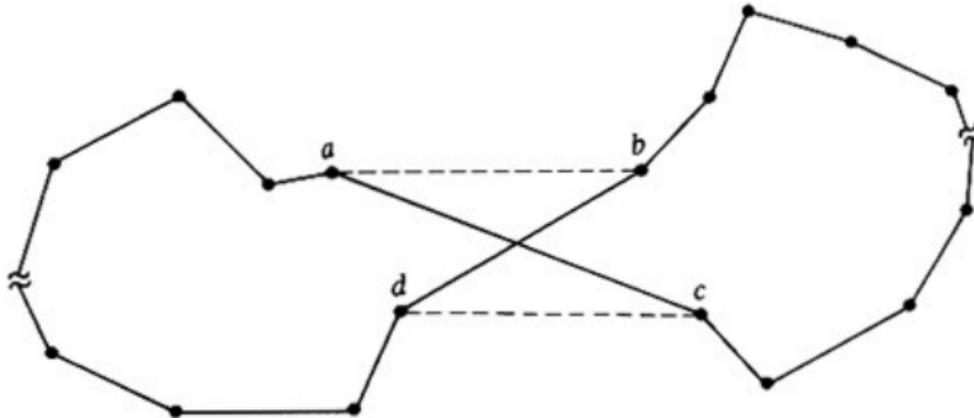
**FIGURE 6.26** The traveling salesman tour can be improved by substituting the intersecting links  $(a, c)$  and  $(b, d)$  by  $(a, b)$  and  $(c, d)$ .
