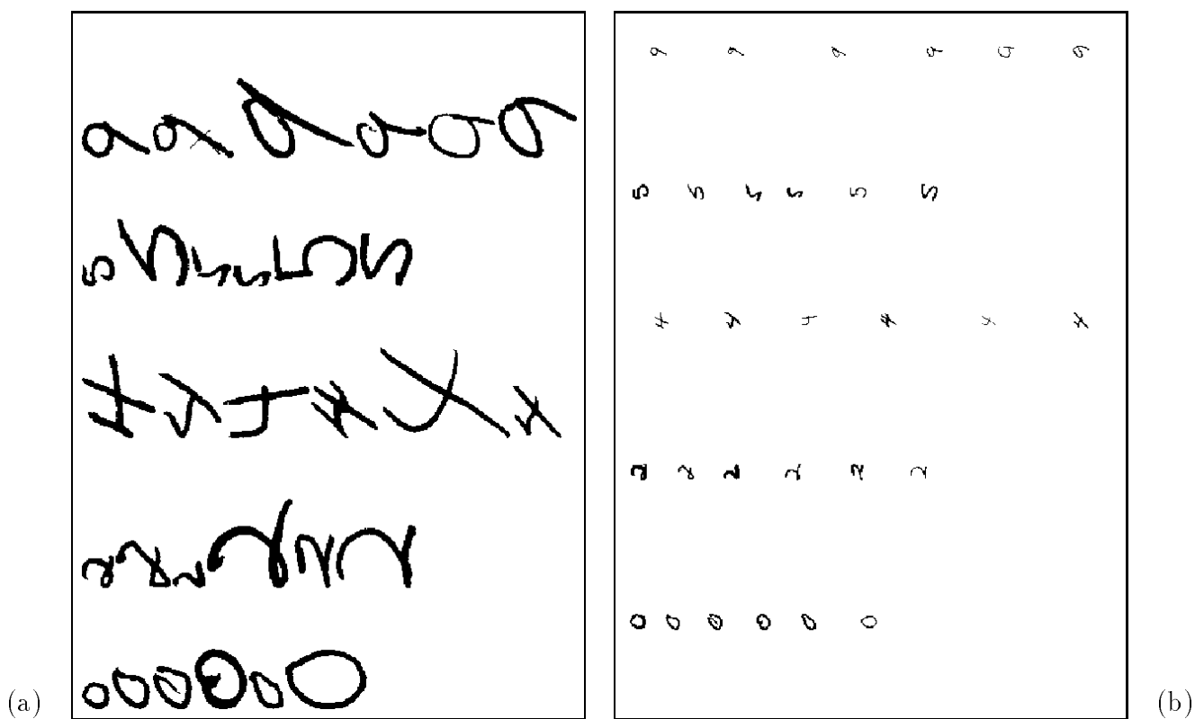
Figure 7: Examples of training patterns before (a) and after (b) size normalization. Figures have the same scale.
